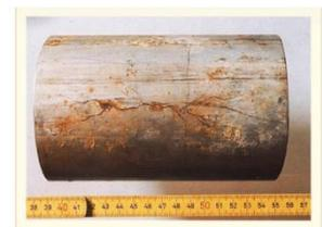
Stress corrosion cracking
